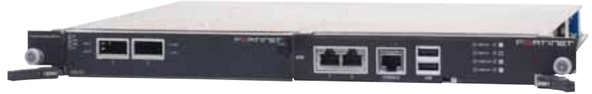
FortiCarrier-5001A-DW Multi-Threat Security Blade (shown with optional ADM-XB2 Module)
